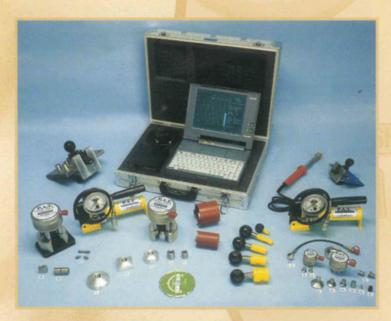
Digital logger where the test results are documented in graphical diagrams and statistical form. The test samples may be presented in a variety of formats with arithmetic averages, histograms, standard deviation etc.
